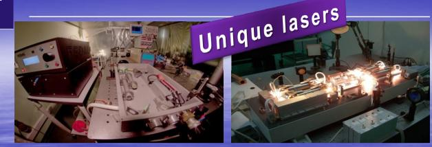
diode-pumped solid-state lasers for range finding (eye-safe range, high-stable, short-pulse, high brightness, compact, efficient, Q-switched, Yb-Er:Glass)
