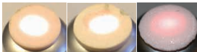
Fig. 2. Translucent samples of glass-ceramics after annealing at temperatures of 800, 1100, 1250 °C for 30 min.
